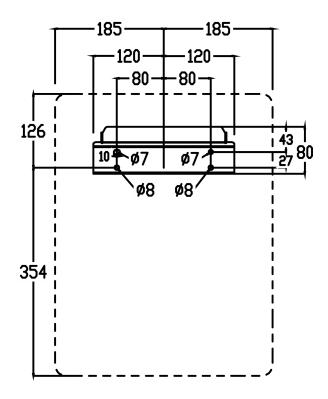
Before drilling holes, please ensure the distance between the machine and nearby objects.
