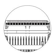
Please keep the top of filter flush with the back of inverter. Please adjust to the position where the lateral fins can be seen from the holes on both sides of the filter according to the figure in which the arrow towards to the wall.
