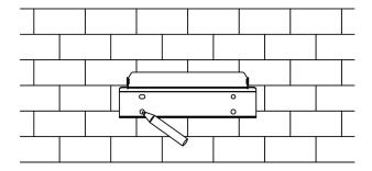
Drill holes with electric drill, make sure the holes are at least 50mm deep and 8mm wide, and then tighten the expansion tubes.
