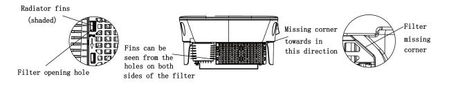
Press the filter down from the top. Check if all fins are covered by filter. Ensure that the filter is installed and secured in right position.
